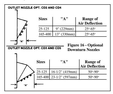
Unit heaters may be specified with optional downturn air nozzles to direct the discharge tempered air. The nozzles are shipped separately for field assembly and installation. The horizontal louvers are removed from the heater and re-installed into the outlet of the downturn nozzle.
